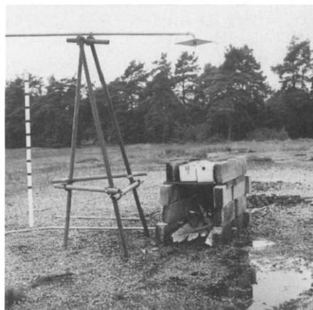
Fig. 2. Hearth and sprinkler system.
